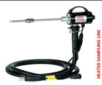
With heated, easy replaceable glass wool filter With exchangeable probe tube and gas temperature measurement using K-type thermocouple
