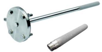
Low dust sampling probe with filter
