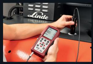
The Bosch-Soot number is being determined with the Densitometer, which is connected to the NOVA plus remote control unit.
