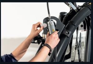
A heated probe prevents condensation during soot measurement.
