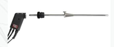
**Gas sampling probe** for industrial combustions, unheated, without filter for short, complete emission monitoring including NO2/SO2, probe handle for exchangeable tubes, with 9 foot gas sampling line (VITON)
