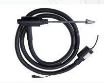
**Heated gas sampling probe** with heated sampling line, length 9 foot, 266°F temperature regulated Gas temperature measurement using K-type thermocouple. With heated, easy replaceable guartz wool filter.
