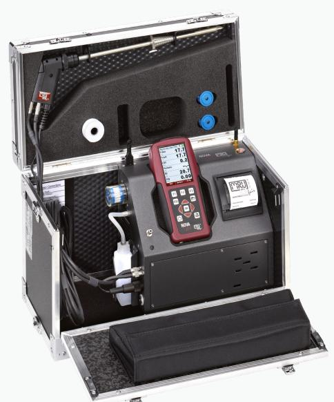
Remote control unit in comfort edition also usable as a separate measuring instrument eg. for pressure, temperature, leakage detection and more
